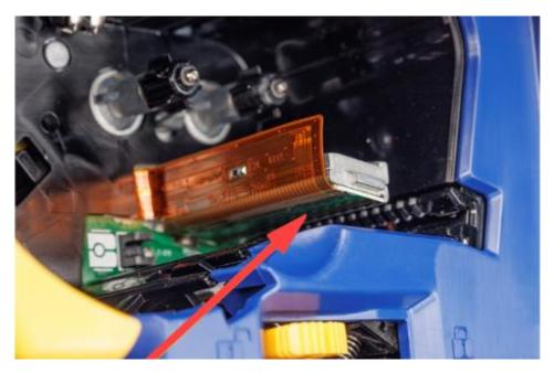
4. With the same moistened swab, gently brush the **platen roller**. You may need to lock the printer to access more of the platen roller.
